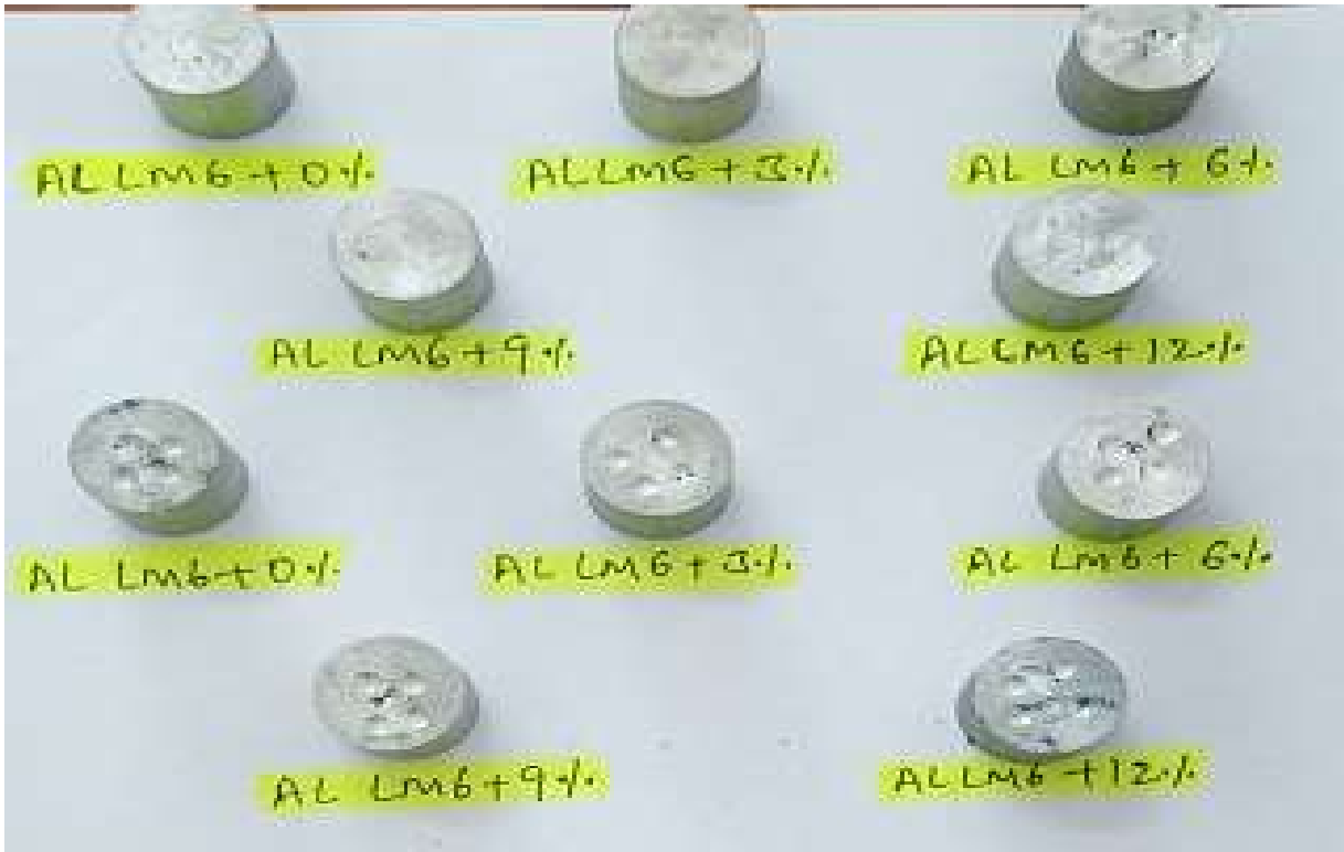
Figure 10: Hardness Test Samples Before and After Indentation.
