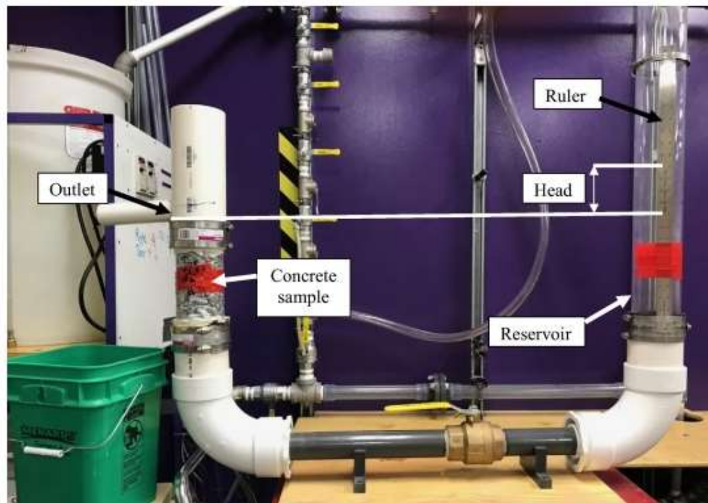
Figure 3: Falling head permeability test apparatus.[14]
